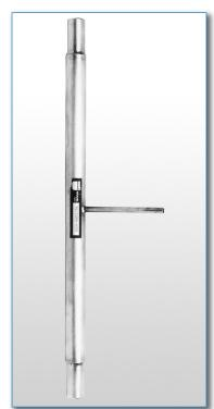
Model 7610 is the basic Mott IGS filter. The porous metal element is mounted in a housing with all-welded construction for maximum reliability. This design allows minimal hold-up volume and provides connections suitable for compression fittings. The IGS filter can be used in gas sampling applications in positive pressure systems without an eductor (see Bypass Filter arrangement on the next page).
